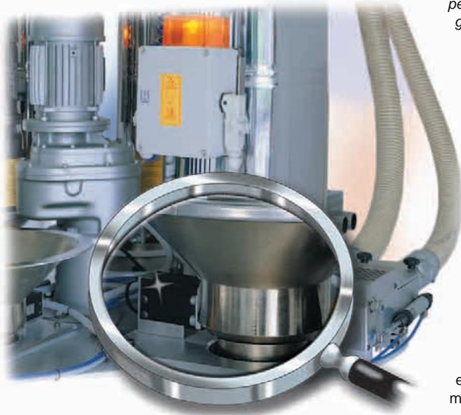
*The system is based on installing the common feeder on a load cell. Every cyclone is equipped for loading 2 materials. The load cell weighs the first material that enters inside the cyclone; when the required weight is reached, the load cell activates a valve to load the second material etc. Once the total weight is reached it falls into the mixer and is mixed for at least 7 minutes.*
