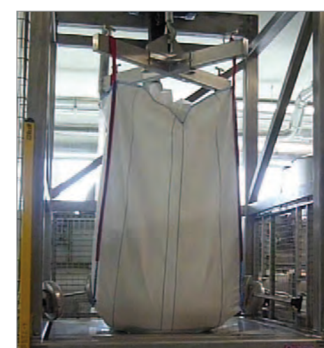
PNEUMATIC PISTONS WITH DIRECT ACTION TO THE BULK BAG TO FACILITATE THE UNLOADING PROCESS
