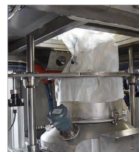
1) OPENING PNEUMATIC TIGHTENING SYSTEM FOR DUST PROOF BULK BAG DISCHARGING
