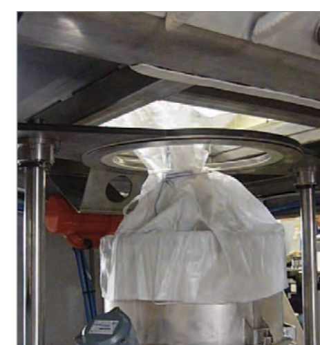
1) OPENING PNEUMATIC TIGHTENING SYSTEM FOR DUST PROOF BULK BAG DISCHARGING
