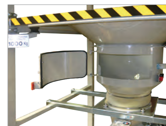
WIDE HATCH FOR SAFE BULK BAG OPENING
