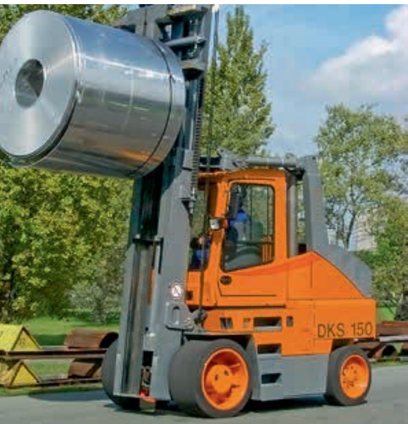
Chariot frontal compact charges lourdes, 12 – 15 t, au choix moteur diesel ou gaz Carrello elevatore compatto per carichi pesanti, portata 12 – 15 t diesel o gas
