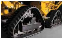
QUAD TRACK ADVANTAGE. The optional quad track system offers improved floatation, reduced surface damage, increased tractive effort and greater stability.
