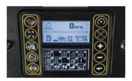
KNOWLEDGE ON DISPLAY. An integrated display allows the operator to optimize machine performance by adjusting operating attachment and ground drive parameters using machine diagnostic information — including engine rpm, fuel level, battery voltage, engine coolant temperature and engine hours.
