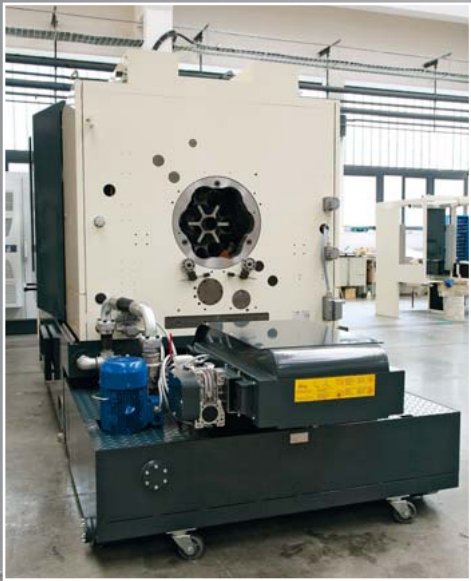
Mobile sedimentation tank inserted into the machine base – traditional solution by the TAJMAC-ZPS
