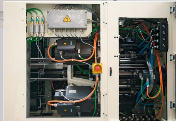
Tandem arrangement of drive sections: – section of drives of axial tools – section of drives of longitudinal slides – section of drives of spindles
