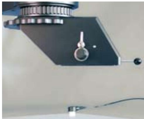
*The adjustment of the working angle is easily accessible using the small lever on the side*
