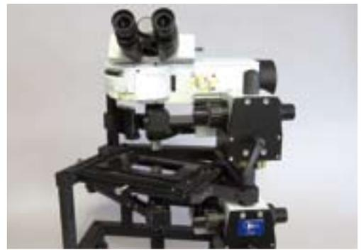
*Split field Microscope for top and simultaneous bottom view together with a laser inspection*
