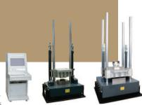
The hydraulic lifting vertical shock tester is used to simulate the shock applied on the product in the actual environment, to assess the function reliability and the integrity of the structure of the product in the shock environment. This equipment is used for the conventional half-sine wave, post-peak sawtooth wave, square wave, and shock response spectrum function etc. impact tests.
