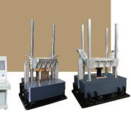
Pneumatic vertical shock and bump test system is a shock and bump test equipment featuring with the novel design, high degree of automation, simple operation and easy maintenance. This equipment is used for the conventional half-sine wave, post-peak sawtooth wave, square wave, and impact response spectrum function etc. shock tests.
