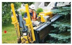
NARROW WHEN NEEDED. With a slender profile, the D9x13 S3 can easily maneuver within narrow jobsites and yard gates. To enhance sidehill stability and ease loading and unloading, the tracks extend 6.5" (16.5 cm) outward, adding up to 18% more width (at the tracks).
