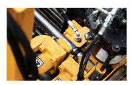
**SHORTEN CYCLE TIMES.** Due to reduced hydraulic flow restriction to the rear vise clamp and rotation cylinders as well as valve sequence improvements, vise speed has been increased to help shorten cycle times and improve productivity as compared to previous models.
