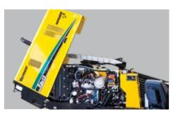
SERVICEABILITY. A one-piece, hinged hood offers durability as well as easy access to key service points.
