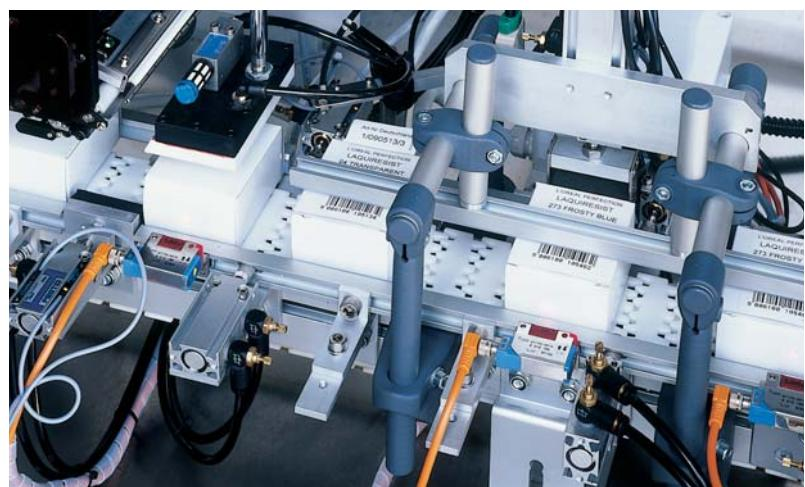
contact labelling of products moving at high speed
