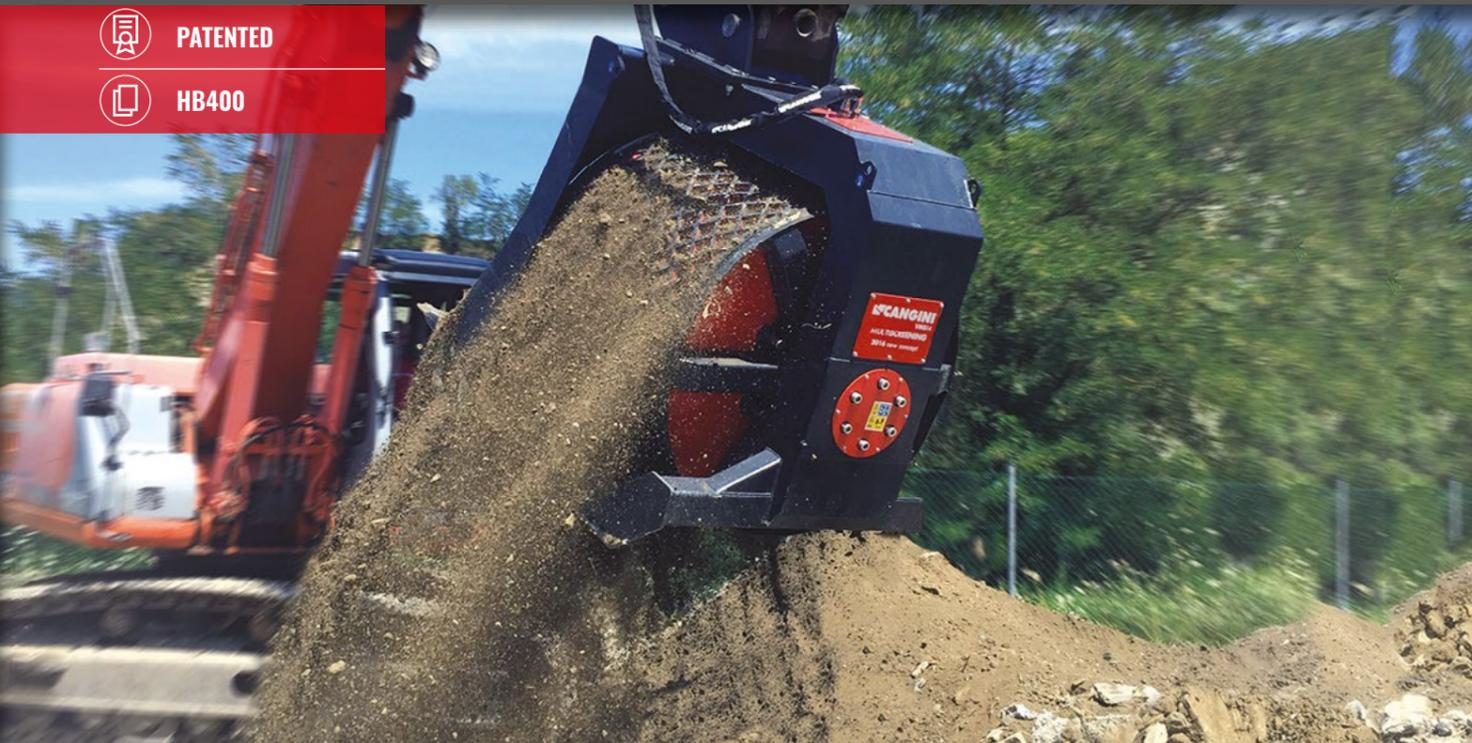
LE NOUVEAU GODET, ET SON NOUVEAU SYSTÈME AVEC DOUBLE PANIER ROTATIF PROJETÉ POUR MACHINES JUSQU'À 35 TONNES, EST ADAPTÉ AUX TRAVAUX DE CRIBLAGE SUR TERRAINS REMUÉS. LA TAILLE DU MATÉRIAU SÉLECTIONNÉ - DE 25 À 60 MM (65 MM POUR LE VMS20-VMS30) - PEUT ÊTRE VARIÉE DIRECTEMENT ET HYDRAULIQUEMENT DE LA CABINE, SANS REMPLACER AUCUN ÉLÉMENT MÉCANIQUE EN RÉDUISANT LES TEMPS DE TRAVAIL.
