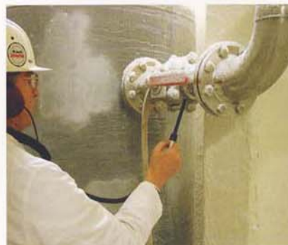
Picture above Leak detection by an air sound detector
