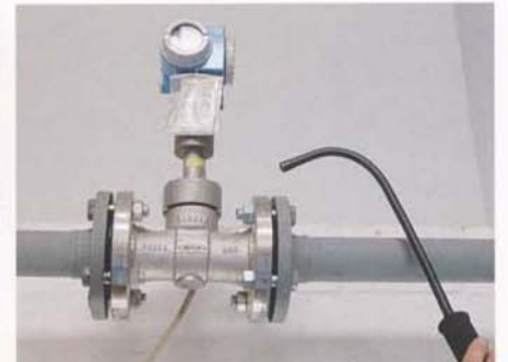
Pictures below a telescope bar offers a wide range for location of leaks (maximum length 3 m 9 8 feet), large mobility by using a flexible probe
