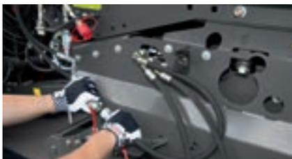
Desserrez le raccord hydraulique
