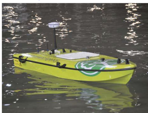
Raccordement proue Compartiment batteries Puits ADCP Coffre arrière
