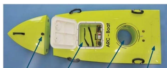
Raccordement proue Compartiment batteries Puits ADCP Coffre arrière
