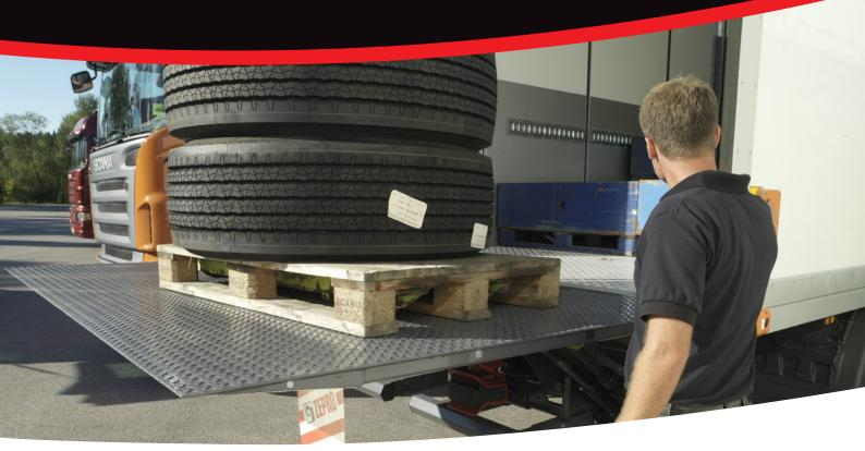
Special lift for vehicles with underslung tow hook. Includes three-piece underrun protection. Frame mountings supplied separately. The frame is bolted to the drawbeam to save space. Lifting capacity of 1500 and 2000 kg.
