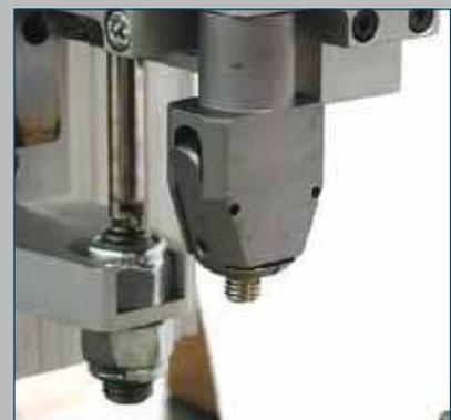
The photo shows a special head for holding screws for flat screw M8 with ratio length screw/diameter head equal to 0,9 and installed on triple-stroke slide.
