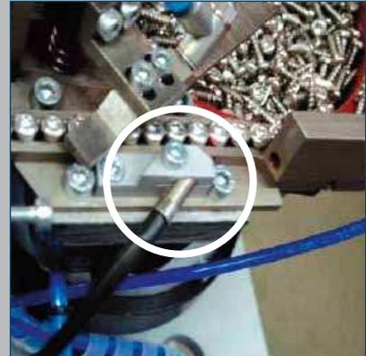
The photo shows an application of a Fiam overload sensor with optical fibre
