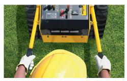
VZ STEERING. Instead of additional levers and steerable wheels, the operator can turn the machine using only the handlebars. These bars also provide additional leverage when operating in difficult terrain.
