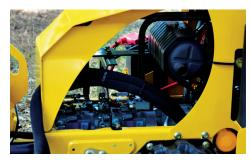
**OPERATORS, START YOUR ENGINE.** The 25 hp (18.6 Kw) Kohler electronic fuel-injected (EFI) gasoline engine offers improved fuel economy reducing greenhouse gas by an average of 25% as compared to conventional carbureted engines. And, best of all, makes choke cables obsolete. Simply put, it's time to start your trencher like you would your car.
