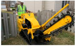
SLENDER PROFILE DESIGN. A 34.5" (87.6 cm) width makes the unit fit through tight areas and narrow gates.
