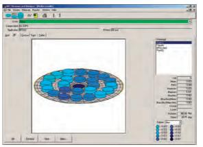
Malvern Panalytical's SuperQ software makes it simple to set up spot patterns for uniformity measurement over the full surface area of wafers up to 300 mm.
