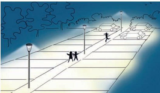
Optic 5068 - square: this light distribution is designed for lighting squares, parks, car parks, public spaces, etc. Only available for 32 LED version.
