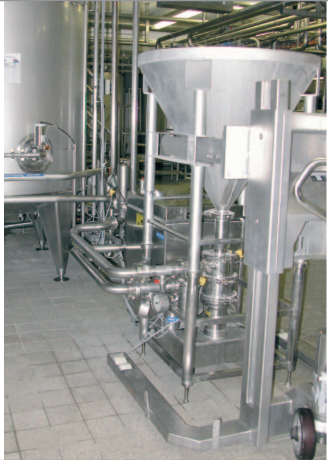
YTRON-ZC in the Dairy Industry Application: Dispersing of a Protein Hydrolysate
