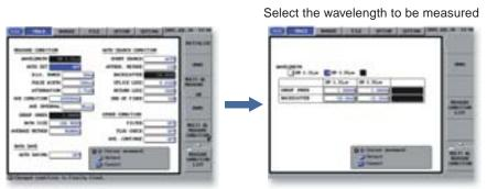
Multi Wavelength Continuous Measurement is a function that allows you to switch the wavelength being measured while keeping the same measurement conditions. This is convenient when you need to measure two wavelengths in a single fiber.
