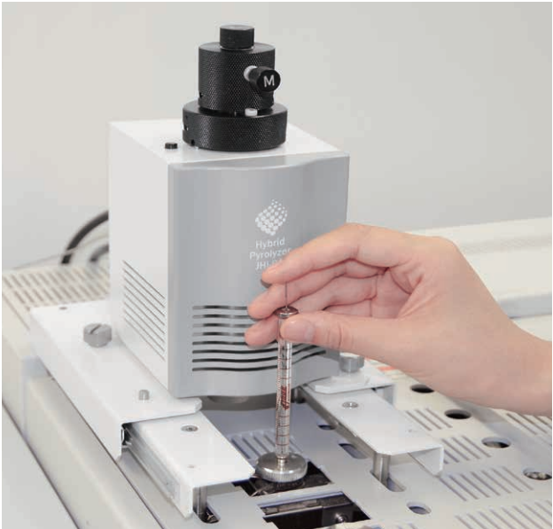
The pyrolyzer can slide backward.
