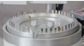
Turntable with Pyrofoils. Turntable for sample cups also comes as a standard accessory.
