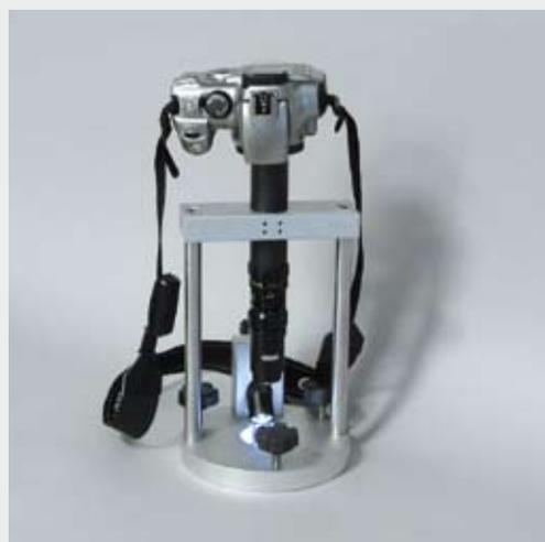
Portable Zoom with mount for C-Mount or digital SLR cameras and battery operated illumination
