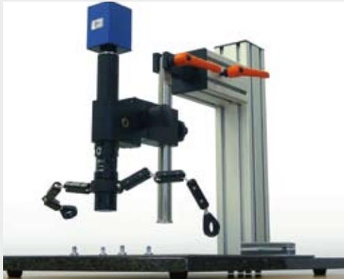
Mounting a High-Speed microscope performing quality checks in a production line
