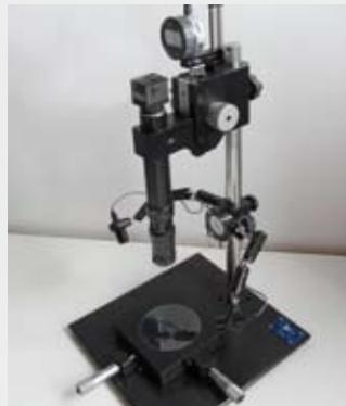
Measuring system for height measurements with manual measuring stage (→ page 26)
