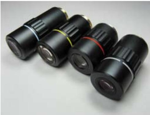
Optimised for use with Automated Analytical Microscopes, Infinity-Corrected Objectives achieve significantly higher magnifications and increased resolutions. The objectives provide a high quality plain achromatic design. All objectives feature standard M26 x 36T (Mitutoyo thread) threads for a wide compatibility.
