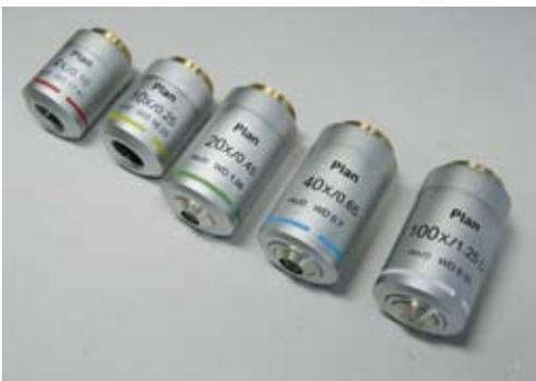
These objectives have an optimal price and performance ratio and come with a standardised RMS-thread and a correction length of 45 mm. The 20x, 40x and 100x are spring-loaded to prevent damage. Oil Immersion is recommended for the 100x objective.
