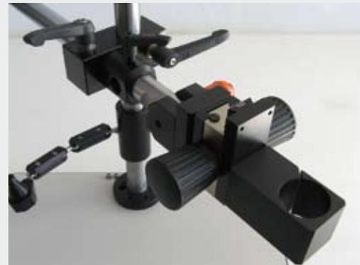
Totally flexible setup for a TV microscope used in a laboratory
