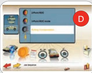
(EN) **«RUN-OUT» COMPENSATION PROGRAMS:** Available 3 different programs to compensate «Run-Out» problems on tyre and rim and possible mistakes caused by an incorrect rim-clamp coupling: 2 and 3-point ROC by rotation the clamp of 180° and push mode ROC which eliminates the need to lift the vehicle.
