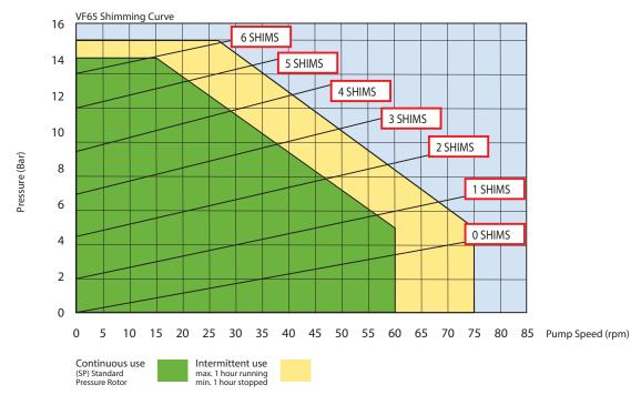
For product temperatures above 65°C and/or viscocity above 2000 mPas use one shim less than shown
