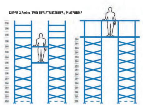
CASE "A" Two tier structure with suspended walkways CASE "B" Platform with continuous floor
