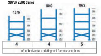
SUPER-ZERO uprights and frames are allowed with the use of SUPER-ZERO beams and shelves, only. Bay lengths 900/1050/1200 mm only, with a max. load capacity of 200 daN per shelf, for uniformly distributed loads.
