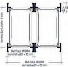
When designing two tier structures, consider the dimensions and details of the sketch shown above. Always refer and adhere to the calculation and safety code summarized on pages 4 and 5.
