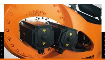
Two motors and gear units in axis 2 and a new drive concept in axis 1 ensure maximum accuracy with heavy payloads.
