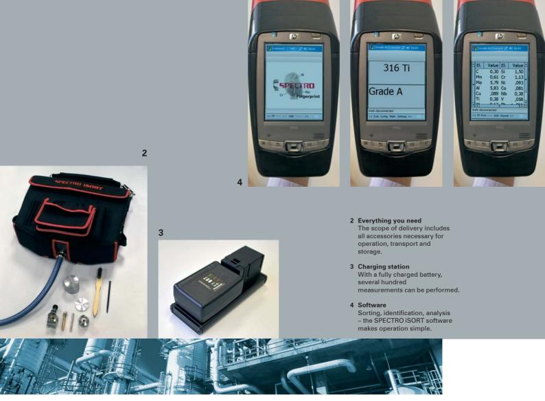
The **software** enables sorting, grade identification and grade verification as well as determination of the elemental composition. It fulfils all expectations for modern, intuitive and simple operation while remaining easy-to-learn. Program modules for data processing, evaluation and documentation round out the program.
