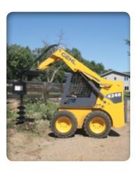
POWERVIEW® LIFT ARM provides strength, durability and excellent view of the tires and sides of the loader for increased safety.
