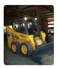
compact machine width as narrow as 48.4 inches (1229 mm) and overall height just over 70 inches (1786 mm) on the 3640E.
