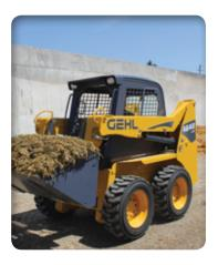
ACCELERATE RAPIDLY with maintenance-free, radial-piston drive motors with high start-up torque and maximum ground speeds up to 11.9 mph<sup>1</sup> (19.2 km/hr).
