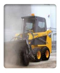
provide up to 10.1 gpm (38.2 L/min) of standard hydraulic flow for powering a wide variety of attachments.
