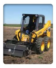
STRONG HYDRAULICS with standard flat-faced couplers provide a high hydraulic flow up to 16.5 gpm (62 L/min) to power a variety of attachments.
