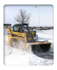
EXCEPTIONAL HYDRAULICS up to 30 gpm (114 L/min) with optional high-flow power a wide variety of attachments and produce outstanding attachment performance.
