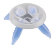
Rotor angulaire | GDF011 5 mL×4 12000 rpm/9660 ×g
