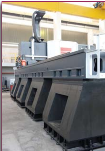
Epoxy concrete columns
