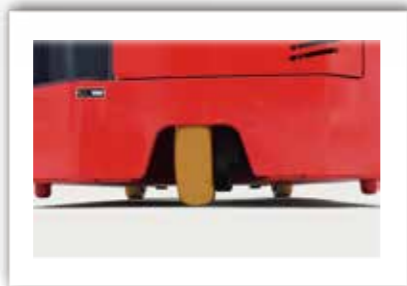
3-pivot design, with better stacking stability
