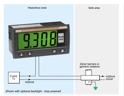
The BA308E loop powered 4/20mA indicator is a fourth generation instrument that is electrically and mechanically compatible with the earlier BA308C, but has a much larger full 4 digit display providing maximum visibility from a 144 x
