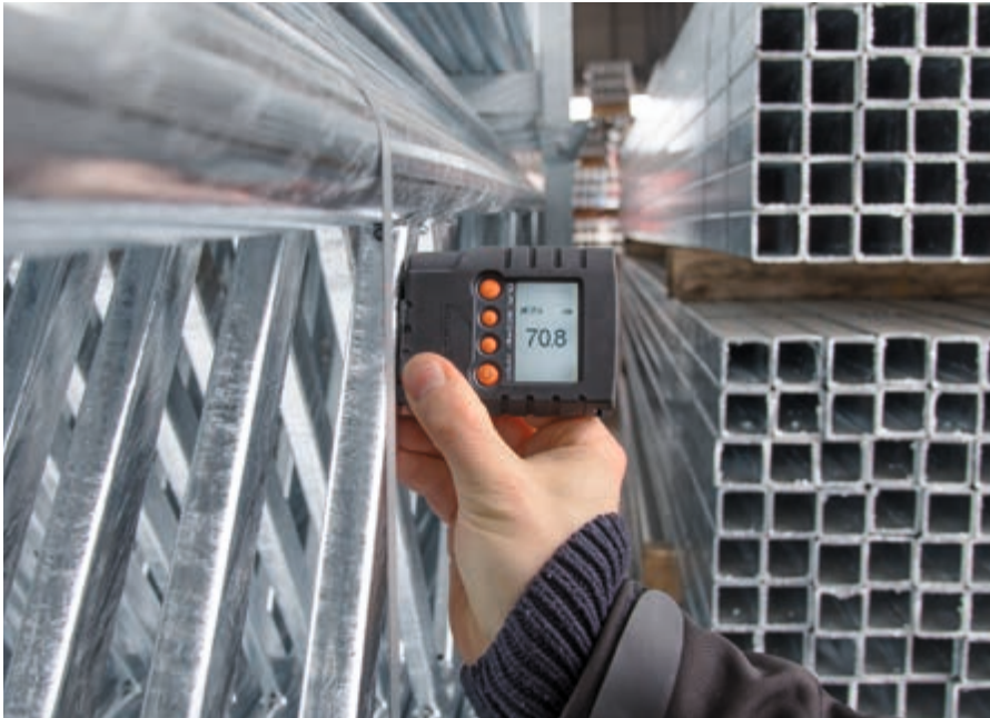
The lit display rotates automatically, allowing easy readout in any measurement position
