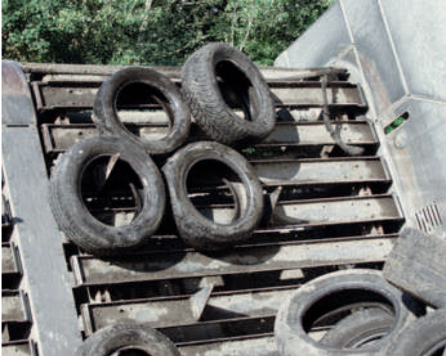
A hook lifter separates the total tires for a controlled and continuous feeding.
