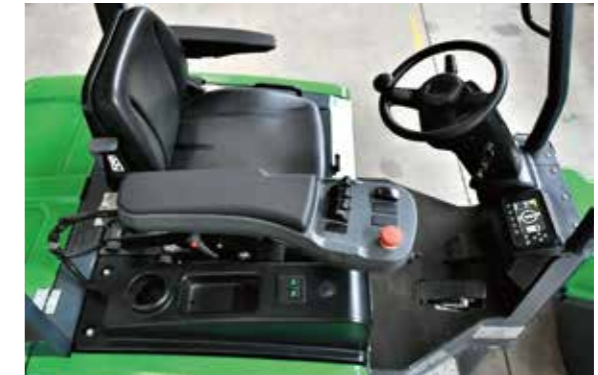
Options:Electric proportion integrated handle, easier operation and more accurate
