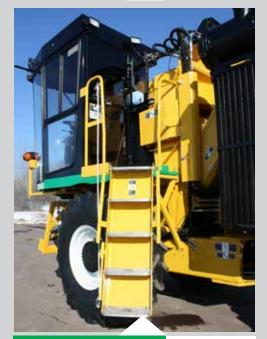
Easy access ladder: New design for operating mode. Simply flip locking lever up and pull ladder out of the way.
