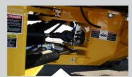
Articulating chassis: Rear wheels track with front wheels for easier, more responsive steering for sharp turns and handling rough field conditions
