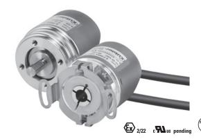
The Sendix F36 multiturn is an optical multiturn encoder in miniature format, without gears and with 100% insensitivity to magnetic fields. With a size of just 36 x 42 mm it offers a shaft or a blind hollow shaft of up to 10 mm.
