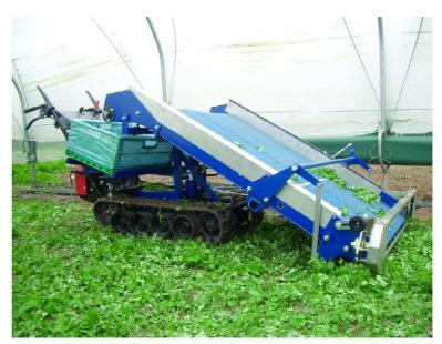
is fed into trays at the rear, while an operator at the side drives the larger self-propelled machines.
