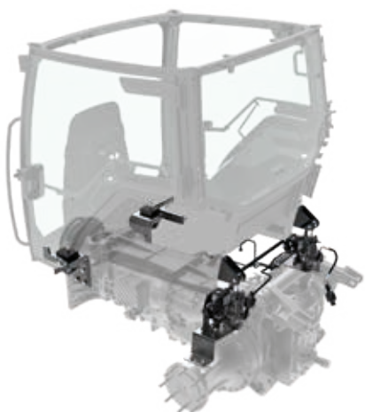
• Suspension hydraulique semi-active
