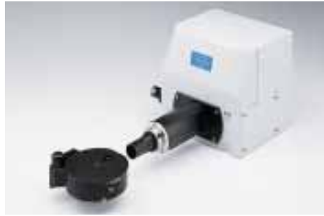
Scanning unit for IX81 inverted microscope Dedicated mirror unit cassette is required.
