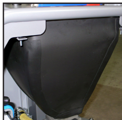
Insulated pellet hopper with 23 kg (50.7 lb) capacity
