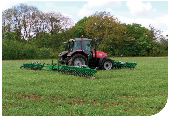
For larger systems, split front to rear systems give improved weight distribution
