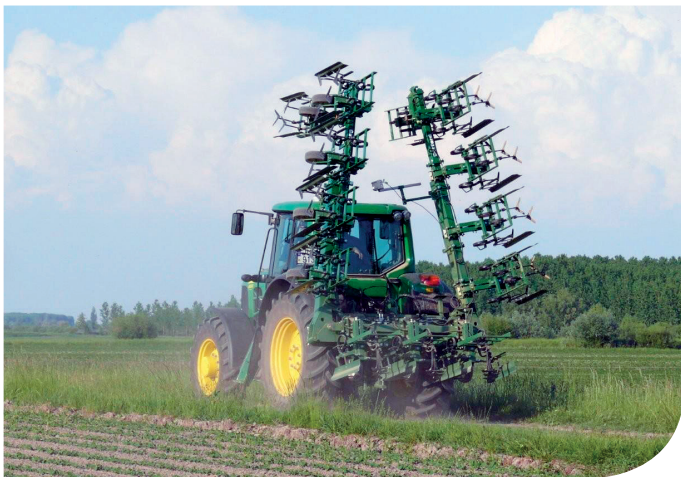
4.5 metre to 18 metre hydraulic folding frames
