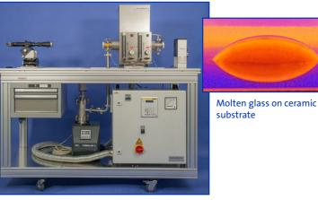
High temperature contact angle measuring system with vacuum or inert gas OCA 25-HTV 1800
