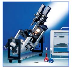
Analysis of the roll of angle with an OCA 25 and electronic tilting base unit TBU 95
