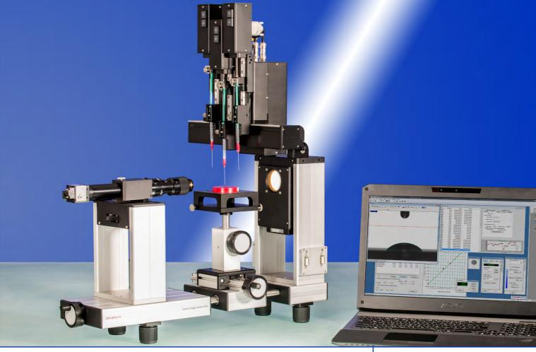
Determination of the surface free energy with an OCA 25 with electronic direct dosing system DDE/3 and three ESr-D
