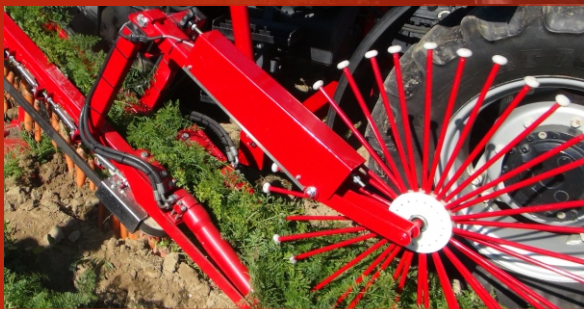
Hydraulic driven rotary dividers
