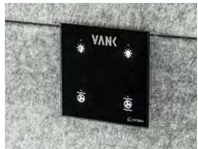
A 4-button touch pad with stepless lighting adjustment, stepwise ventilation adjustment. Optionally, a 6-button touch pad PA-6 with stepless lighting adjustment, stepwise ventilation adjustment, and an occupancy sensor.
