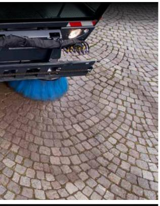
With the optional, autonomous brush control system, the angle of the disc brushes can be hydraulically adjusted to the road conditions from the driver's cab. Ground pressure on each disc brush can also be adjusted individually from the driver's cab. This makes it even easier to thoroughly sweep out right-angled corners, gutters and hard-to-reach areas.
