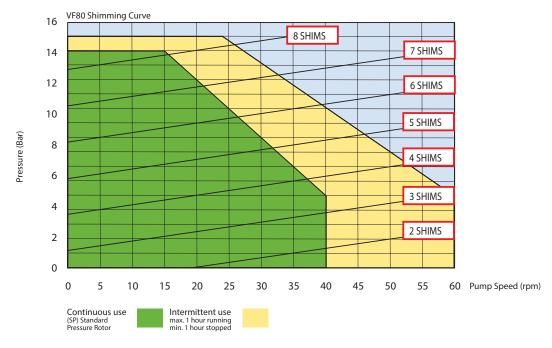
For product temperatures above 65  $^{\circ}\text{C}$  and/or viscocity above 2000 mPas use one shim less than shown
