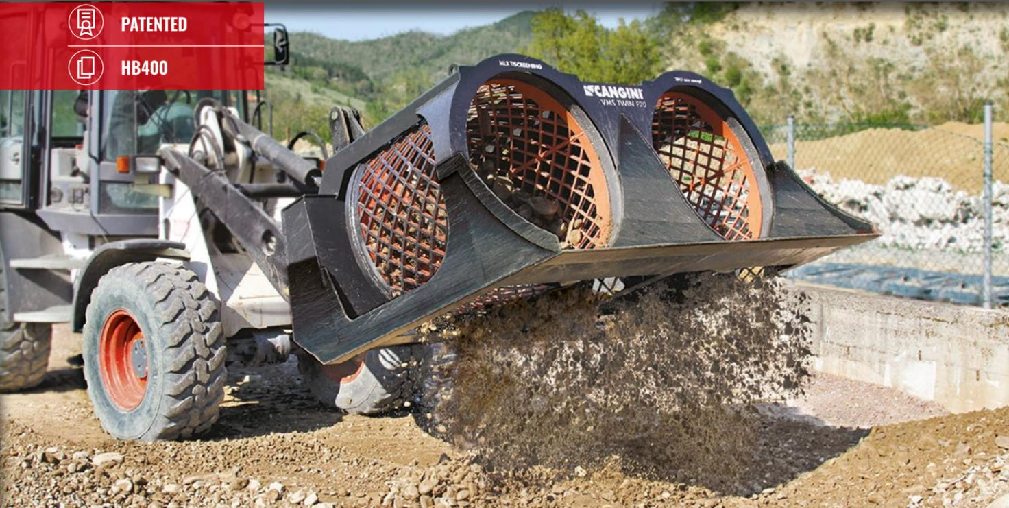
LE NOUVEAU GODET MULTISCREENING DOUBLE, ET SON NOUVEAU SYSTÈME AVEC DEUX DOUBLES PANIERS ROTATIFS JUMELÉS DANS UN SEUL CHÂSSIS, PROJETÉ POUR ACCOUPLEMENT FRONTAL, EST ADAPTÉ AUX TRAVAUX DE CRIBLAGE SUR TERRAINS REMUÉS. LA TAILLE DU MATÉRIAU SÉLECTIONNÉ - DE 25 À 60 MM - PEUT ÊTRE VARIÉE DIRECTEMENT ET HYDRAULIQUEMENT DE LA CABINE, SANS REMPLACER AUCUN ÉLÉMENT MÉCANIQUE EN RÉDUISANT LES TEMPS DE TRAVAIL.
