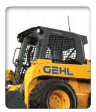
**EXCELLENT VISIBILITY** to the sides, rear and front is achieved with a unique, low-profile boom design. A roof window allows the operator to view the lift arm when in the fully raised position.
