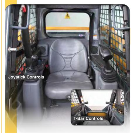
GET IN CONTROL – Joystick controls, hand/ foot controls or mechanical T-bar controls provide the ultimate in operator comfort.
