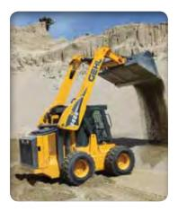
VERTICAL-LIFT boom design delivers extended reach and high lift heights for easy truck loading and material handling.
