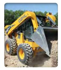
HEAVY-DUTY CHASSIS provides excellent weight distribution, enhancing machine stability. A rear bumper and counterweight on the model V330 GEN:2 add protection and towing capability.
