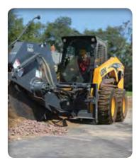
AUXILIARY HYDRAULICS are standard, powering many attachments. Optional high flow increases this capability. Dependent on control pattern, a rocker switch or foot pedal provides electronic proportional flow control.
