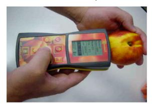
In fruit and vegetables establishing the optimal harvest time is a crucial issue, since fruit shelf-life potential and quality are closely related to the ripening stage at harvest. The DA Meter is a very promising tool both for practical and scientific applications, since it allows to monitor on-tree fruit ripening (as well on the same fruit), to establish accurately the optimal harvest time and it can be used in cool store to establish maturity changes as well.
